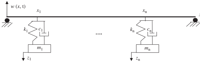
Fig. 2. Beam equipped with absorbers.
